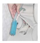
Take complete pump and flush tube out the water tank
