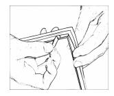
Start applying the seal first at both corners of the toilet. Then divide the remaining length along the back.
