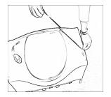
Finally, cut the seal at length
