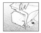
Start removing the protection sheet off the tape at the back side of the toilet.
