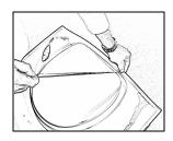
Remove the protection sheet off the tape at the left & right side of the toilet. For the sides, start removing the sheet at the free hanging end of the seal at the bottom.
