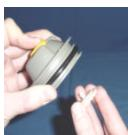
E. Place vent plug back into the waste tank and turn the two arrows back to each other
