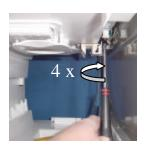
Screw the mechanism back on its place.
