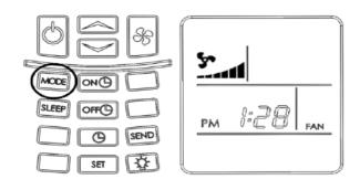
Press the fan speed key, high/medium and low speed are available in succession.
