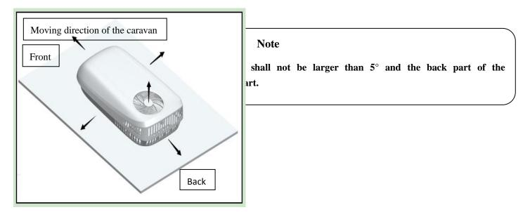
• The left lower figure shows the minimum clearance distance required between the BELAIRE air-conditioner and any obstructions on the roof.
