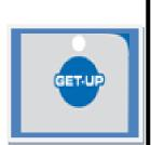
Press GET UP to release the jacks from the ground. They stop at the point of pivoting. At this point eventually used spacers must be removed. You will hear intermitted beeps from the system. Pressing again GET UP the jacks go to the driving position.
