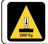
Use fixing points with sufficient stability. Consider every jack can lift up to 2500 kg. If necessary the fixing points at the chassis must reinforced with adequate parts.
